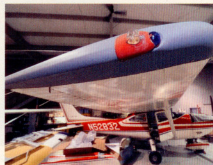
A job this big calls for lots of paperwork (far left). Air Mod's Dennis Wolter (above) puts the final touches on a soundproofing insert. New fiberglass wing tips were installed (left).
