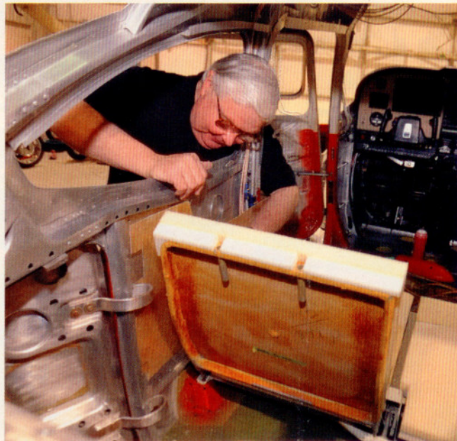
A job this big calls for lots of paperwork (far left). Air Mod's Dennis Wolter (above) puts the final touches on a soundproofing insert. New fiberglass wing tips were installed (left).
