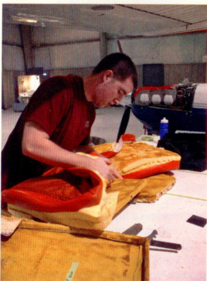
The old seat covering material was yanked (left) while new leather-covered interior door panels were installed to the door inserts (below). Cracked fuel-line connections at the wing roots (bottom left) were replaced with new rubber sleeves. New seat rails from MacFarlane Aviation Inc. were installed (bottom right) to prevent seat slips.
